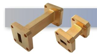
The HASCO WR-42 Millimeter Waveguide Straight Section **HWSS42-2.0-ES** operates from 18 GHz to 26.5 GHz. This WR-42, K-Band waveguide straight section is constructed with a Square UG-595/U Flange.
