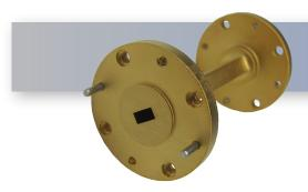
The HASCO WR-19 Millimeter Waveguide Straight Section **HWSS19-2.0-ER** operates from 40 GHz to 60 GHz. This WR-19, U-Band waveguide section is constructed with a Round UG-383/U-M Flange.
