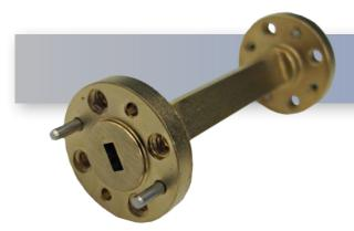
The HASCO WR-15 Millimeter Waveguide Straight Section **HWSS15-2.0-ER-1** operates from 50 GHz to 75 GHz. This WR-15, V-Band waveguide section is constructed with a Round UG-387/U-M Flange.
