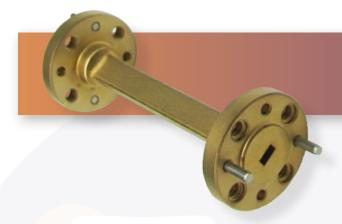
The HASCO **HWSS06-4.0-ER** is a WR-06 Millimeter Waveguide Straight Section that operates from 110 GHz to 175 GHz. This WR-06, waveguide section is constructed with a Round UG-387/U-M Flange.
