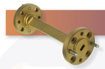
The HASCO **HWSS06-3.0-ER** is a WR-06 Millimeter Waveguide Straight Section that operates from 110 GHz to 175 GHz. This WR-06, waveguide section is constructed with a Round UG-387/U-M Flange.
