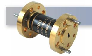
The HASCO WR-15 Millimeter Waveguide Fixed Attenuator **HWFA15-03-1.0** is rated to 0.3 Watts and operates from 50 GHz to 75 GHz. This V-Band, WR-15 attenuator has a fixed attenuation value of 3 dB at center frequency and is constructed with a round UG-385/U Flange.
