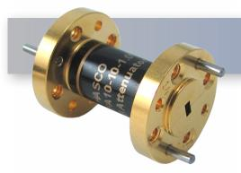
The HASCO WR-12 Millimeter Waveguide Fixed Attenuator **HWFA12-10-1.0** is rated to 0.3 Watts and operates from 60 GHz to 90 GHz. This E-Band, WR-12 attenuator has a fixed attenuation value of 10 dB at center frequency and is constructed with a round UG-387/U Flange.
