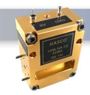
The HWLNA10-W10045 is a Full W-Band Low Noise Amplifier with a gain of 20 dB from 75-110 GHz. The Full Band Noise Figure is 4.5 dB typical. This LNA Bias operates with 7-12VDC. Internal reverse bias protection ensures reliability. This is an excellent full W-Band LNA for receivers, Down-Converters, and general lab use.
