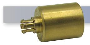
The HASCO **HT6SMPMF** is a push on RF Load Termination from HASCO. This RF Load Termination will operate up to 6 GHz and rated for 1 Watt. The SMPM termination was developed for dense connector application, 5G requirements and high speed simiconductor testing.
