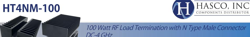
The HASCO **HT4NM-100** is an RF termination (also called RF load or dummy load) that operates from DC to 4 GHz and handles up to 100 Watts (CW). Our Type N termination/load has a male gender. HT4NM-100 Type N termination offers 1.15:1 max VSWR DC-3GHz and 1.25: 1 VSWR at 3-4 GHz. The HASCO 100W Type N termination has a heatsink body which is designed to provide adequate heat dissipation within its full frequency of operation.
