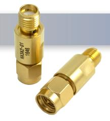
10 dB - Fixed Attenuator SMA Male To SMA Female Up To 3 GHz Rated To 2 Watts with Gold Plated Brass Body
