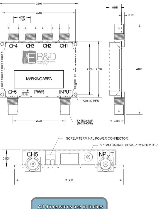
All dimensions are in inches with a tolerance of  $\pm 0.020^{\circ}$
