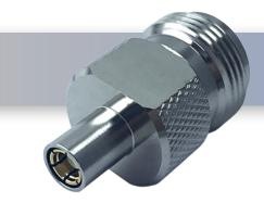
The HASCO SMBP-NJ-FF is an RF Push-On Between Series Adapter that operates from DC to 6 GHz and handles a minimum of 500 mating cycles. Our SMB to N Type Adapters offer 1.20:1 max VSWR.
