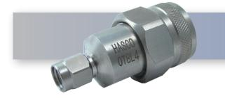
The HASCO **NP-SMAP-MM-01** is a Type N Male to SMA Male Straight RF Precision Adapter that operates from DC to 18 GHz. and offers 1.15:1 max VSWR.
