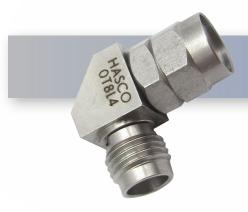
The HASCO **185P-185J-RA** is a 1.85mm Male to 1.85mm Female in-series adapter from HASCO. This in-series 1.85mm to 1.85mm right angle coax adapter will operate up to 67 GHz. Adapters that have a male to female or plug to jack configuration are known as "connector savers." Typically, a low loss or low VSWR male to female adapter is placed on more expensive component connectors to prevent damage.
